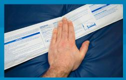
Firmly place pressure on the pad and then release. A long beep from the monitor will indicate it has been synchronized with the pad.
